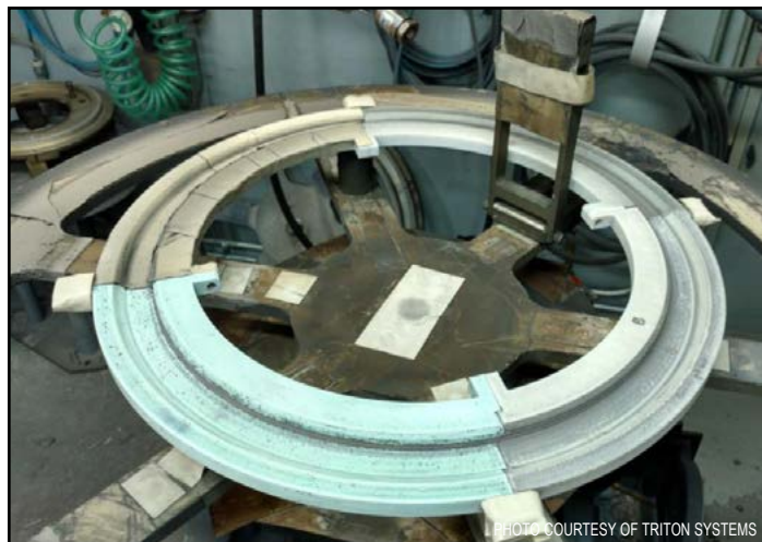
During an Air Force SBIR | STTR project, Triton Systems tested the ability of multiple materials to mask a rotating part during a spray application process. The masks were created with a 3D printer and one of the masks is now being used in an Air Force sustainment operation.
